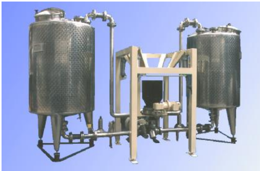
Pic. 1: ystral Conti-TDS with a Big-Bag-station in-between two processing vessels
