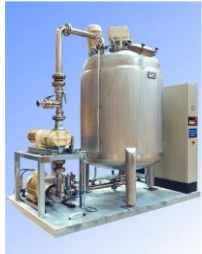
Pic. 4: Conti-TDS with an additional volumetric pump for the production of high viscosity seal compound
