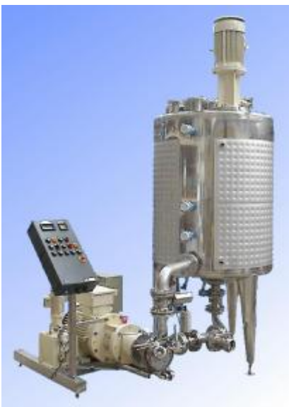
Pic. 8: ystral Conti-TDS in a system for varying batch sizes
