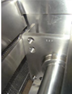
Nibbler's all-welded shaft assembly, 240 grit/0.6 RA internal finish and woven wire stainless steel screen
