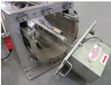
Nibbler's quick release shaft assembly to include the whole basket and front end removed for cleaning
