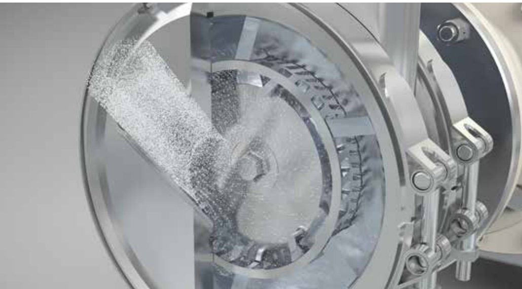
Fig. 1 - Separation of powder particles in the dispersing zone under vacuum pressure
